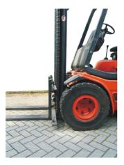
Wear of tyres and elongation of chains lead to a constant lowering of the forks. If the forks touch the ground while the truck is driving, abrasion on the bottom side of the forks will occur.
